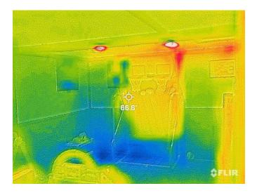
The inspector utilizes infrared thermography to scan the interior of the house, including walls, ceilings, and floors; infrared identifies variances in temperature which may indicate a water penetration issue, e.g. roof leak, plumbing leak, exterior water intrusion, or an electrical concern. These images demonstrate that the inspector performed the infrared scan. Actual issues identified with infrared would be published in the issues section of the report.
